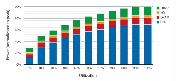
Figure 5.6: Subsystem power usage in an ×86 server as the compute load varies from idle to full usage.
