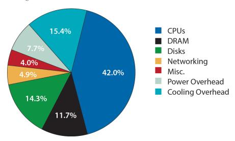
Figure 1.6: Approximate distribution of peak power usage by hardware subsystem in a modern datacenter using late 2012 generation servers and a facility energy overhead of 30%. The figure assumes two-socket x86 servers, 16 DIMMs and 8 disk drives per server, and an average utilization of 80%.
