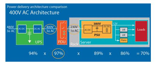
Figure 4.3: Efficiency of 400VAC distribution architecture (Source: Pratt, Kumar, Bross, Aldridge, "Powering Compute Platforms in High Efficiency Data Centers," IBM Technology Symposium, 2006).
