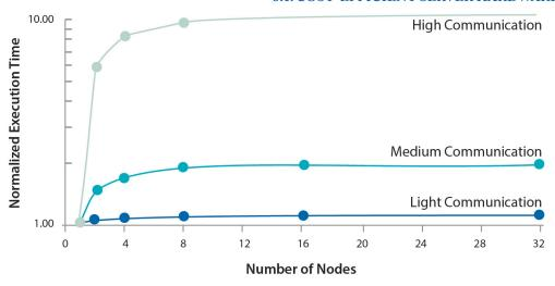
Figure 3.1: Execution time of parallel tasks as the number of SMP nodes increases for three levels of communication intensity. Execution time is normalized to the single node case and plotted in logarithmic scale.
