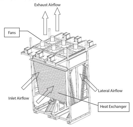
Figure 4.12: Google's "Hot Hut," an in-row, water-cooled fan coil unit.
