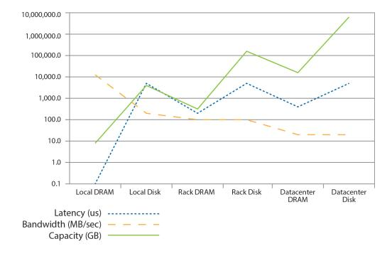
Figure 1.4: Latency, bandwidth, and capacity of a WSC.
