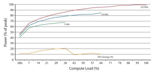
Figure 5.9: Power vs. compute load for an x86 server at three voltage-frequency levels and the corresponding energy savings.
