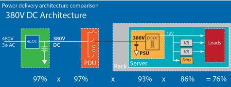
Figure 4.2: Traditional AC vs. DC distribution efficiency (Source: Pratt, Kumar, Bross, Aldridge, "Powering Compute Platforms in High Efficiency Data Centers," IBM Technology Symposium, 2006).
