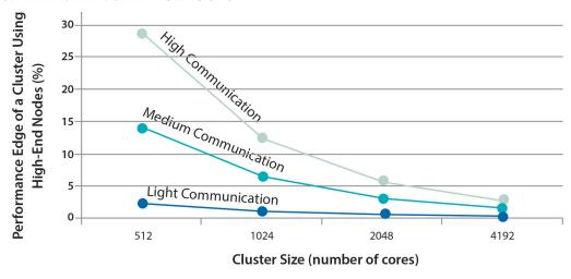
Figure 3.2: Performance advantage of a cluster built with large SMP server nodes (128-core SMP) over a cluster with the same number of processor cores built with low-end server nodes (four-core SMP), for clusters of varying size.
