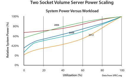
Figure 5.7: Normalized system power vs. utilization in Intel servers from 2006 and 2012 (Courtesy of Winston Sounders, Intel). The green and red lines represent 2006 servers, the two blue ones are 2009 servers, and the orange line is a more recent server. The chart indicates that Intel servers have become more energy proportional in that seven-year period.
